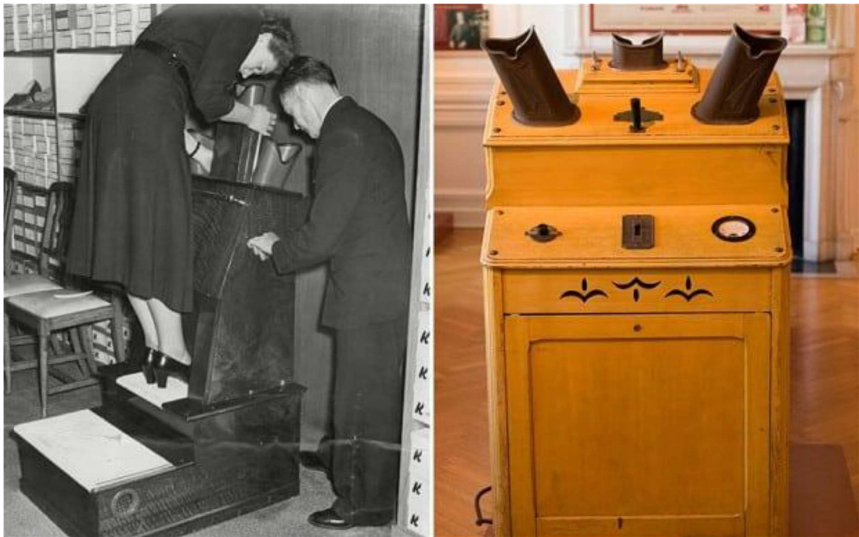
The X-Ray machine known as a Fluoroscope used to measure shoe sizes. Courtesy of ORUA
